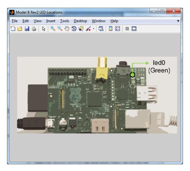
To return the LED to its normal purpose as an indicator of SD card activity, restart the Raspberry Pi hardware.
