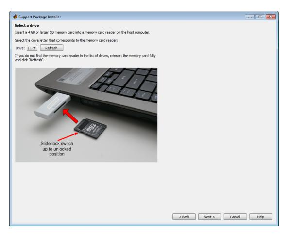
6 Click Write. The installer overwrites all previous data on the memory card with the firmware. This process takes several minutes to complete.
