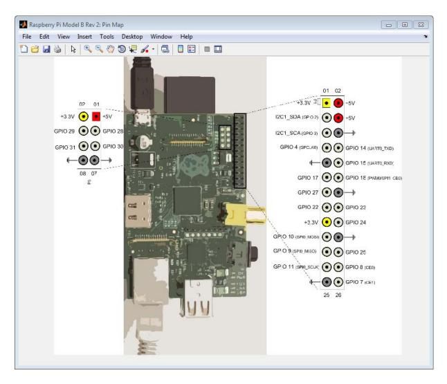
To configure a pin as a digital input, pass an input value to configureDigitalPin.
