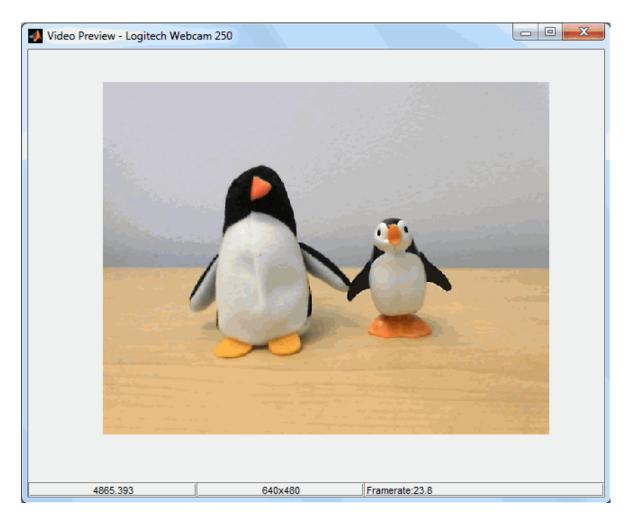
The banner of the preview window shows the camera name. The lower portion of the window shows the timestamp in seconds, resolution, and the frame rate in frames per second. Timestamp is the elapsed time since the object was created.
