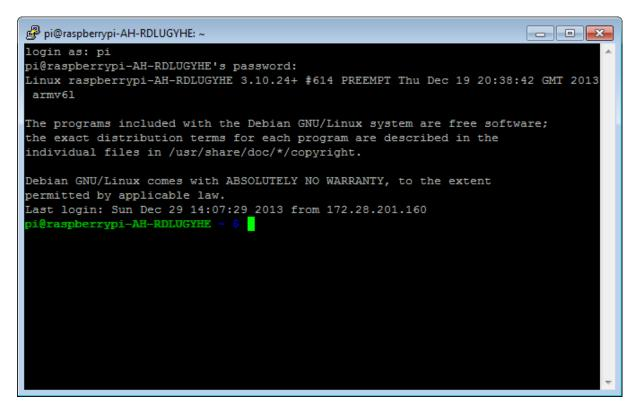
It is a good security practice to change the default password. Use the SSH terminal window to run the raspi-config utility.
