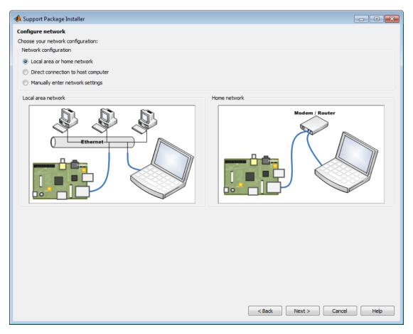
• Direct connection to host computer — Confirm that the Raspberry Pi hardware is connected to your host computer using a direct connection similar to the one that the installer displays. Then, click Next. This option applies static network settings based upon the network settings of the host computer.
