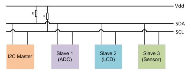
Depending on the model and revision of your board, Raspberry Pi hardware has one or two I2C buses. Each bus has an I2C Master connected to two bidirectional lines, serial data line (SDA), and serial clock (SCL). These two lines are connected to a pair of pins, such as I2C1\_SDA (GPI02) and I2C1\_SCL (GPI03), on the GPIO header.
