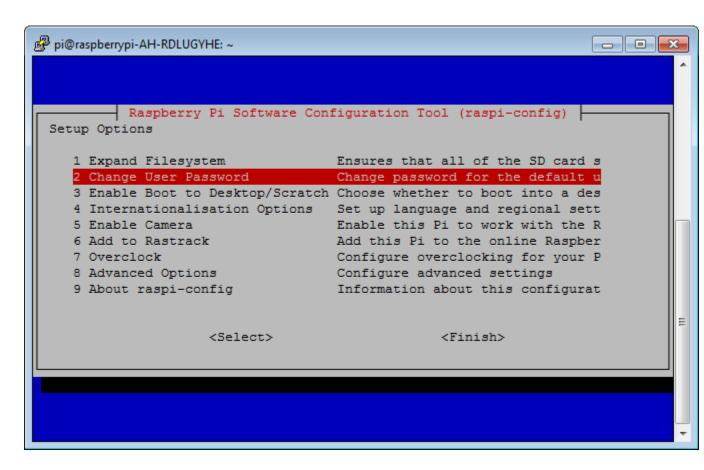
After changing the password, clear the mypi handle and any handles that you created using mypi. Then, use raspi to create a new connection based on the new password.
