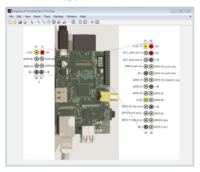
The pin map shows that, for this model and revision of the board, the i2c-1 bus is available on the GPIO header pins I2C1\_SDA (GPIO 2) and I2C1\_SCL (GPIO 3).
