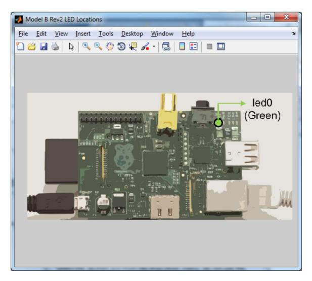
Turn the specified LED on by setting its value to 1 or true.
