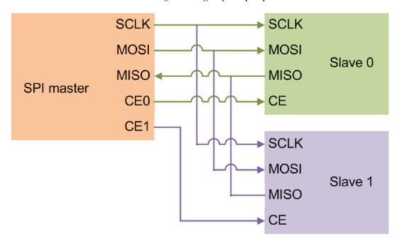
The SPI Master on Raspberry Pi hardware can drive two SPI peripheral device. The SPI Master has four pins:
