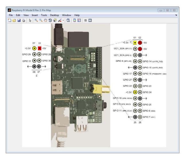
Raspberry Pi hardware uses +3.3V. Do not connect Raspberry Pi hardware directly to devices that use higher voltages.
